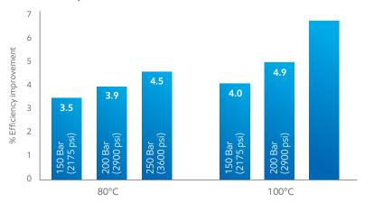
Mobil DTE 10 Excel<sup>™</sup> Series lubricants provided hydraulic pump efficiency benefits up to 6 percent when compared with a typical reference hydraulic fluid in controlled bench testing.
